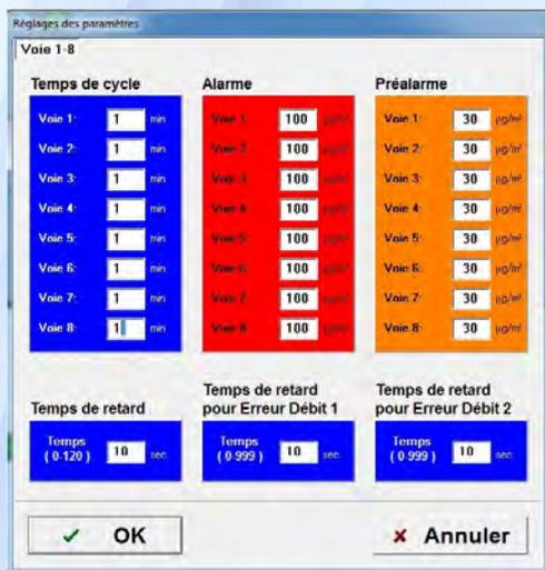
Setting of alarm thresholds
